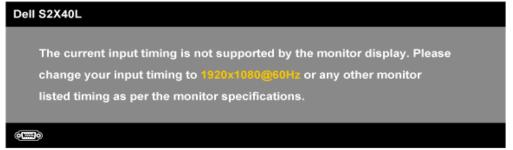
This means that the monitor cannot synchronize with the signal that it is receiving from the computer. See <u>Monitor Specifications</u> for the horizontal and vertical frequency ranges addressable by this monitor. Recommended mode is 1,920 x 1,080.
